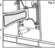
hardware kit (see Fig. 9). Adjust all four nuts evenly. **Do not fully loosen or remove these nuts.**
