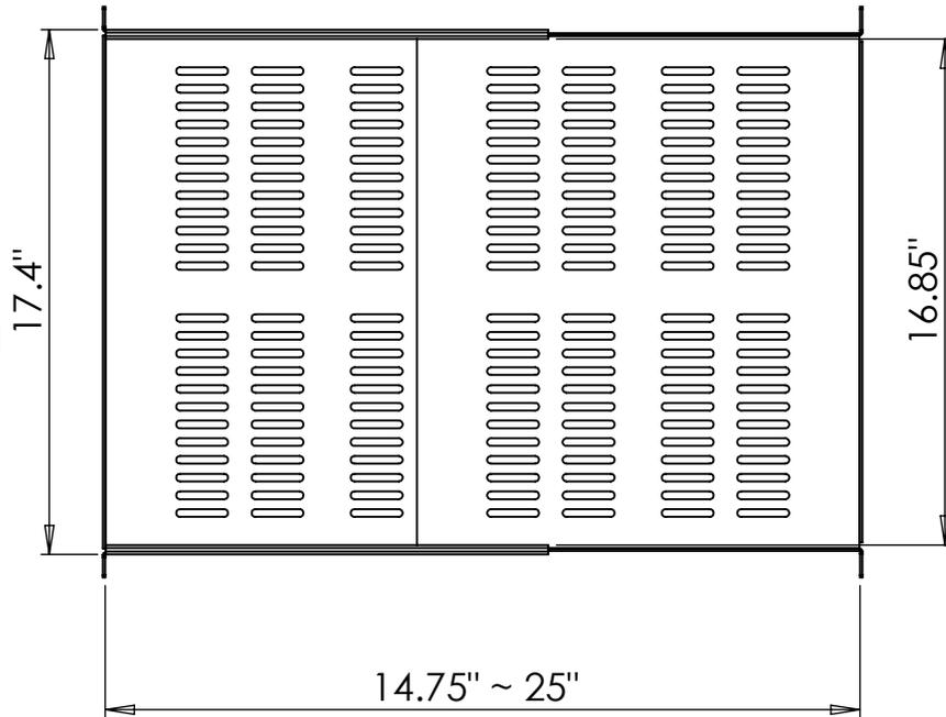
Maximum usable width achieved when mounting the shelf inverted (sidewalls facing down)
