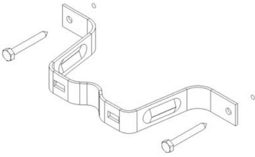
Step 2: Attaching the main support to the mounting surface
