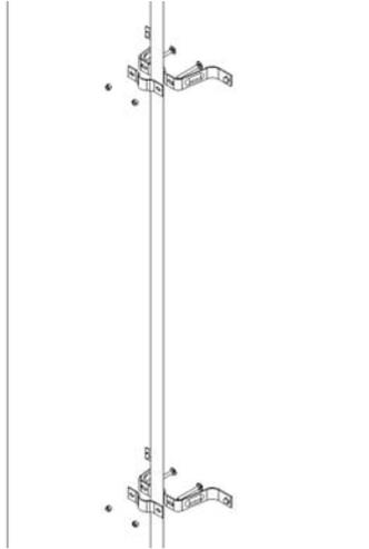
Step 3: Attaching the antenna mast to the main supports
